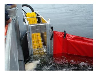
The Lamor Side Collector (LSC-C) is based upon the proven stiff brush oil recovery technology, offers high performance and safety for offshore oil spill recovery operations. The LSC-C is supplied with an outrigger and sweeping boom, which deflect oil and debris from a wide area into the side box for processing. The LSC systems are designed to be used with GTA or MSP pumps.
