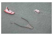
The DESMI RO-KITE is a floating water kite based on a combination of trawl door and ram-air parachute principles. The purpose of this device is to act as a flow powered 'towing vessel' for oil boom systems. This can be either in fast flowing waters or in fast sweeping operations from OSR vessels.
