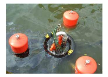
The ALLIGATOR and ARMADILLO belt brush skimmers have a bi-directional belt. In underflow mode (with the belt going down into the oil) the skimmer can achieve a high recovery rate with lighter oils.
