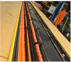
A revolutionary approach to the management of hydraulic & discharge hose systems commonly found between skimmers and power packs. The DESMI ZUH not only enhances safety when dealing with high pressure hoses, but allows for the inspection and replacement of damaged or aged hoses.
